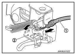
6. Remove hood lock mounting bolts, and then remove hood lock.
