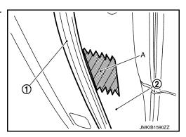
2. Disengage fixing clips on the reverse side of rear door weatherstrip using a remover tool (A).
