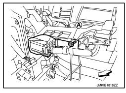
Remove harness fixing clips (A), and then move harness (1) to a location where it does not inhibit work.
