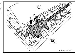
6. In the order of  $1 \to 2$  as shown in the figure, disconnect rod 2 from rod slide hole portion A while pulling handle 1 of glove box lock assembly.
