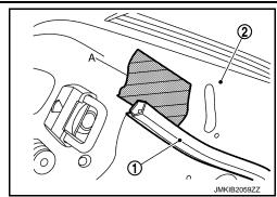
2. Disengage fixing clips on the reverse side of radiator core seal using a remover tool (A).
