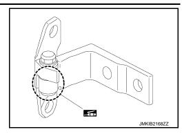
3. Check door check link rotating part for poor lubrication. If necessary, apply body grease.
