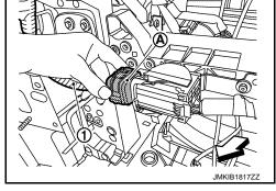
d. Remove mounting bolt (A) of harness bracket.
