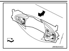
12. Disconnect outside handle cable ① according to the numerical order  $1 \rightarrow 2$  indicated by arrows as shown in the figure from outside handle bracket ②.
