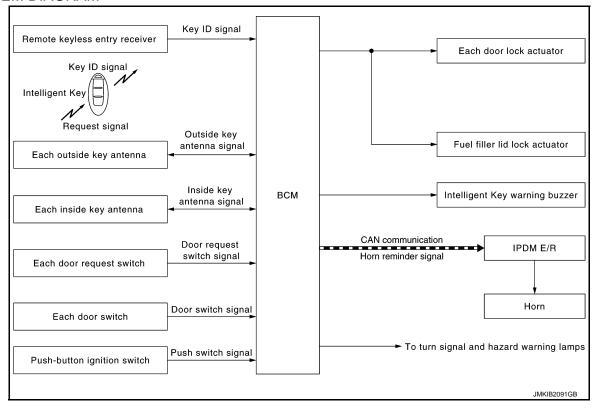
Door lock function controls operation function of the following items.
