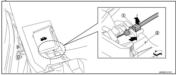
4. Disconnect hood lock control cable (rear) 1 from hood opener lever 2 according to the numerical order  $1 \rightarrow 2$  indicated by arrows as shown in the figure.
