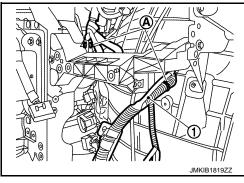
f. Remove fender bracket mounting bolts, and then remove fender bracket LH.
