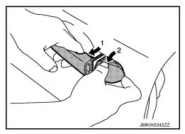
7. In the order of  $1 \rightarrow 2$  as shown in the figure, while pulling outside handle grip ①, slide toward rear of vehicle to remove outside handle grip.
