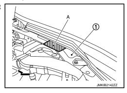
ii. Disengage fixing clips on the reverse side of hood side seal assembly ① using a remover tool (A).
