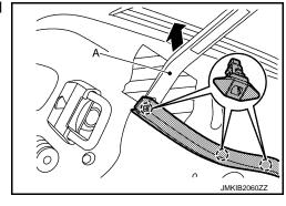
3. Remove radiator core seal.
