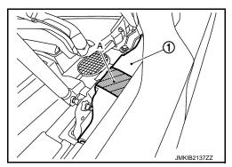
b. Disengage fixing clips on the reverse side of hood side seal assembly ① using a remover tool (A).
