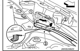
c. Disengage case pawl of hood lock control cable (front) and remove hood control cable protector.
