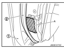
2. Disengage fixing clips on the reverse side of front door weatherstrip using a remover tool (A).
