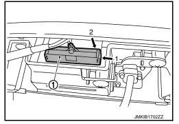
Pinch trunk lid opener request switch from left side (in the direction shown by arrow 3) and disengage tab. Press toward outside (in the direction shown by arrow 4) to remove from trunk lid finisher ②.
