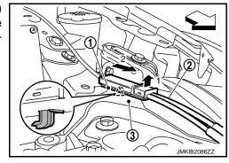
Disengage case pawl of hood lock control cable (front) and remove hood control cable protector.
