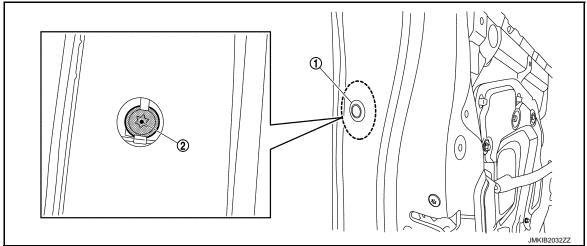
8. In the order of  $1 \rightarrow 2$  as shown in the figure, while pulling outside handle grip ①, remove outside handle escutcheon ②.
