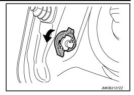
Push fuel lid lock actuator behind the vehicle, while pushing the pawl.
