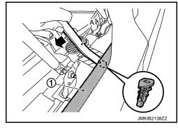
c. Remove fixing clip A, and then remove front fender drip cover 1 according to the numerical order  $1 \to 2$  indicated by arrows as shown in the figure.
