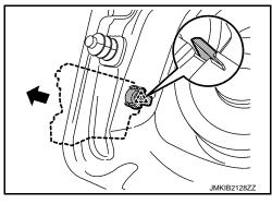
5. Disconnect fuel lid lock actuator harness connector, and then remove fuel lid lock actuator.
