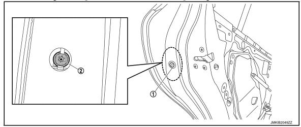
6. In the order of  $1 \rightarrow 2$  as shown in the figure, while pulling outside handle grip, remove outside handle escutcheon.
