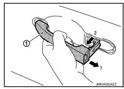
10. Remove front gasket ① and rear gasket ②.
