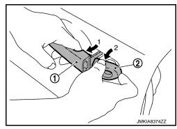
9. In the order of  $1 \rightarrow 2$  as shown in the figure, while pulling outside handle grip ①, slide toward rear of vehicle to remove outside handle grip.
