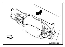
10. Disconnect outside handle cable ① according to the numerical order  $1 \rightarrow 2$  indicated by arrows as shown in the figure from outside handle bracket ②.
