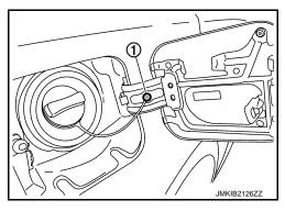
4. Remove fixing screws, and then remove fuel filler lid assembly.
