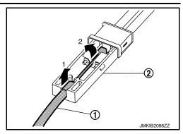
Disengage hood lock control cable (rear) ① fixing pawls, and then remove hood lock control cable (rear) from instrument lower panel ② according to the numerical order 1 → 2 indicated by arrows as shown in the figure.
