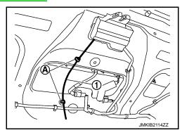
5. Disengage pawls of trunk lid lock cover ①. Open trunk lid lock cover in direction indicated by the arrow as shown in the figure.
