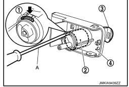
11. Remove sleeve ③ from handle, and then install sleeve to glove box lid lock cylinder ②.
